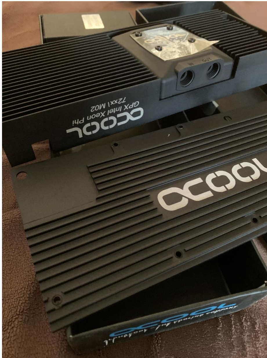
Figure. 1.1.4 [Liquid Cooling for the Xeon Phi Coprocessors]
